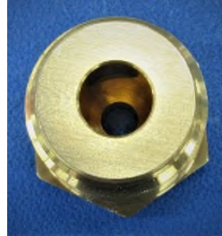
Figure. 3. Incorrect Vent Plug w/o Ball Check & Retaining Pin
