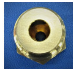
Fig 3. Vent Plug - Missing Ball Check & Retaining Pin
